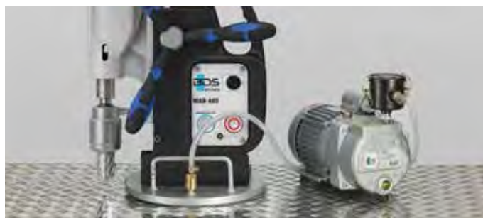
Vacuum plate for smooth corrugated sheet metal/gussets
